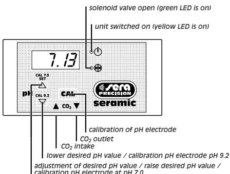
The light-emitting diodes in the controller unit show:
